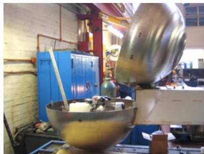
the main sphere of the clock showing electronics hidden inside
